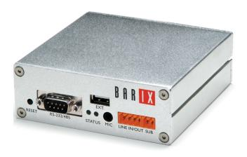
Transmits voice and high quality audio, alarm messages, contact closures and serial data over the network
